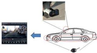
Fig.1 Conceptual car black box system using several camera modules.
