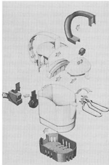
Tea kettle designed for disassembly by Polymer Solutions, Inc., for Great British Kettles Ltd. (From Graedel & Allenby, Industrial Ecology , 1995, page 270)
